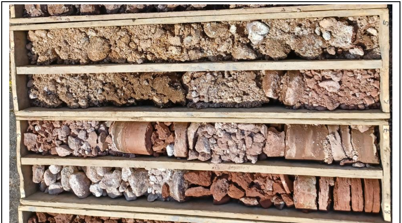
Foto Nr. 8: Kernbohrung KB 41b (4,0 m - 8,0 m)
